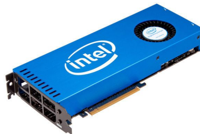
Xeon Phi(s) – (Accelerator and self-hosted)
