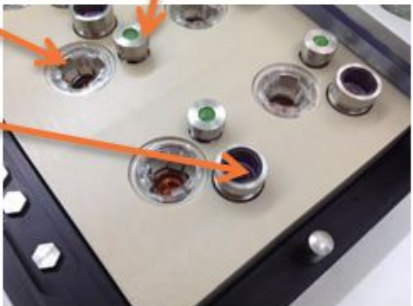
Connects to nanoAnalytics controller for automated TEER monitoring
